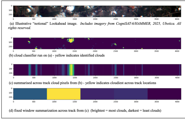
Figure 4. Notional image processing of the lookahead image to drive nadir acquisition targeting. Raw imagery credit Ubotica/Open Cosmos.
