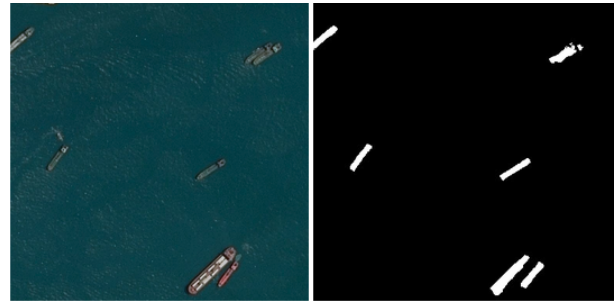
Figure 5. Sample input image and segmented output image for the Ship Segmentation model.
