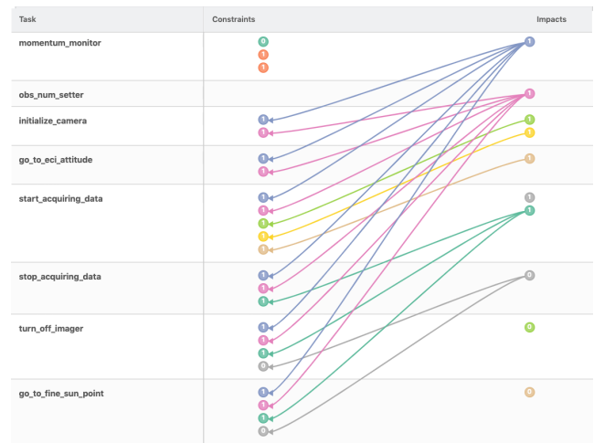
Figure 6: Simplified excerpt of what the constraints and impacts for some of the tasks in the second experiment could look like. This figure was created using a prototype of a tool developed to visualize the relationship between impacts and constraints in a task network.
