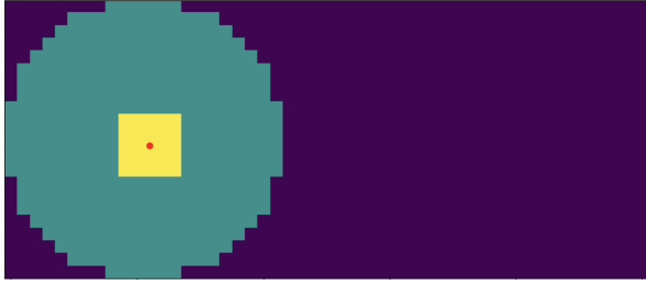
Fig. 4. The reachable range of the primary sensor for a rest-to-rest maneuver with one cycle of slewing time and no computational time reserved, shown in 15 km/pixel resolution. The small red circle shows nadir, which is the starting location of the primary sensor. The yellow area shows the positions that the primary sensor could slew to within one cycle, in the satellite reference frame. The blue area shows the entire range of locations that the primary sensor is capable of slewing to given the 15^\circ maximum off-nadir angle of the primary sensor, in the satellite reference frame. The right edge of the purple area represents the end of the lookahead range.
