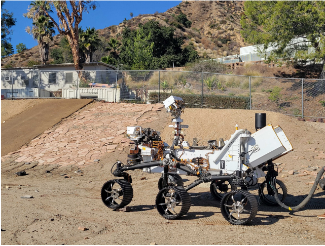
Figure 1. OBP generated plan executing on VSTB in Marsyard 15 November 2022 as part of Super Thread Test 22 (Super TT 22).
