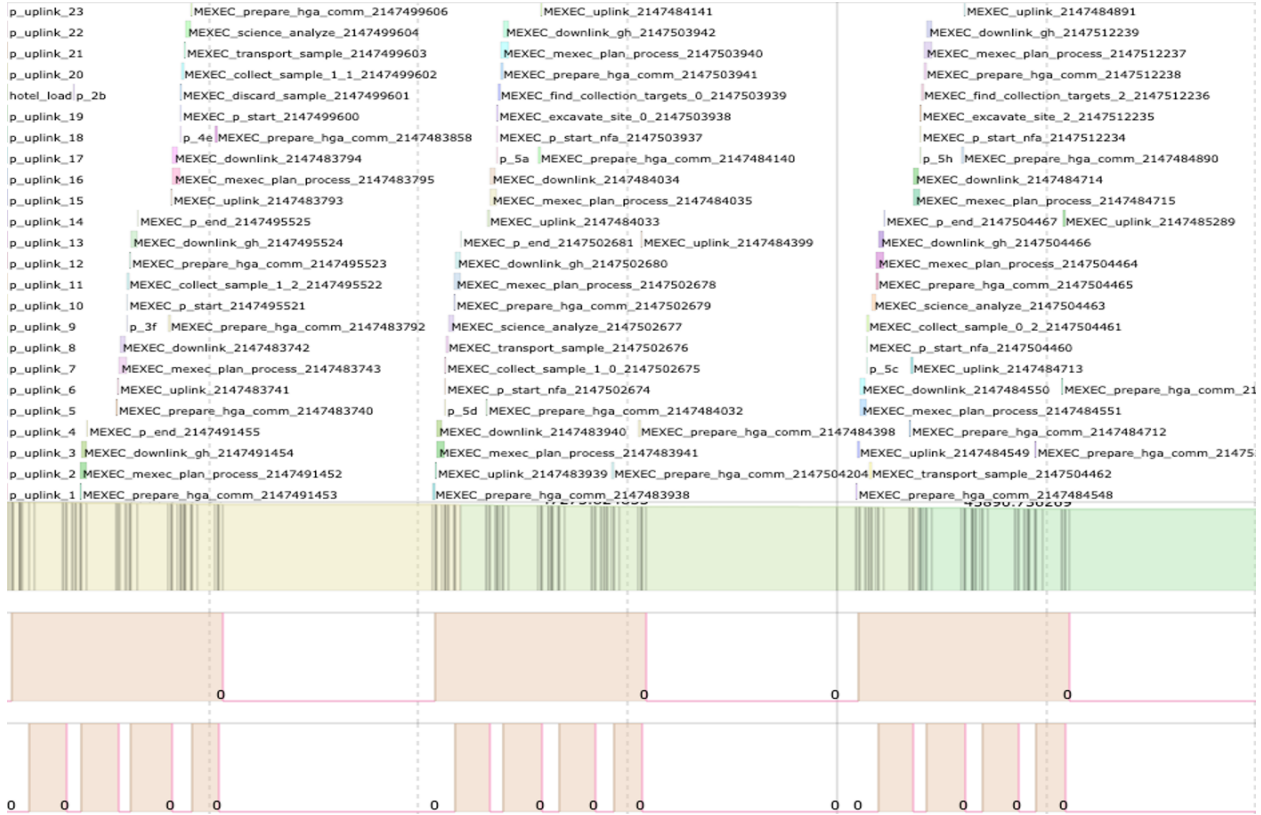
Fig. 8 Sample of a full mission schedule: 3 sites excavated, 9 samples collected over multiple sols, plus episodic imagery, fixed exogenous uplink windows, downlinks. Mission ends when battery depleted.
