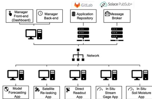
Figure 2: NOS Testbed Architecture
