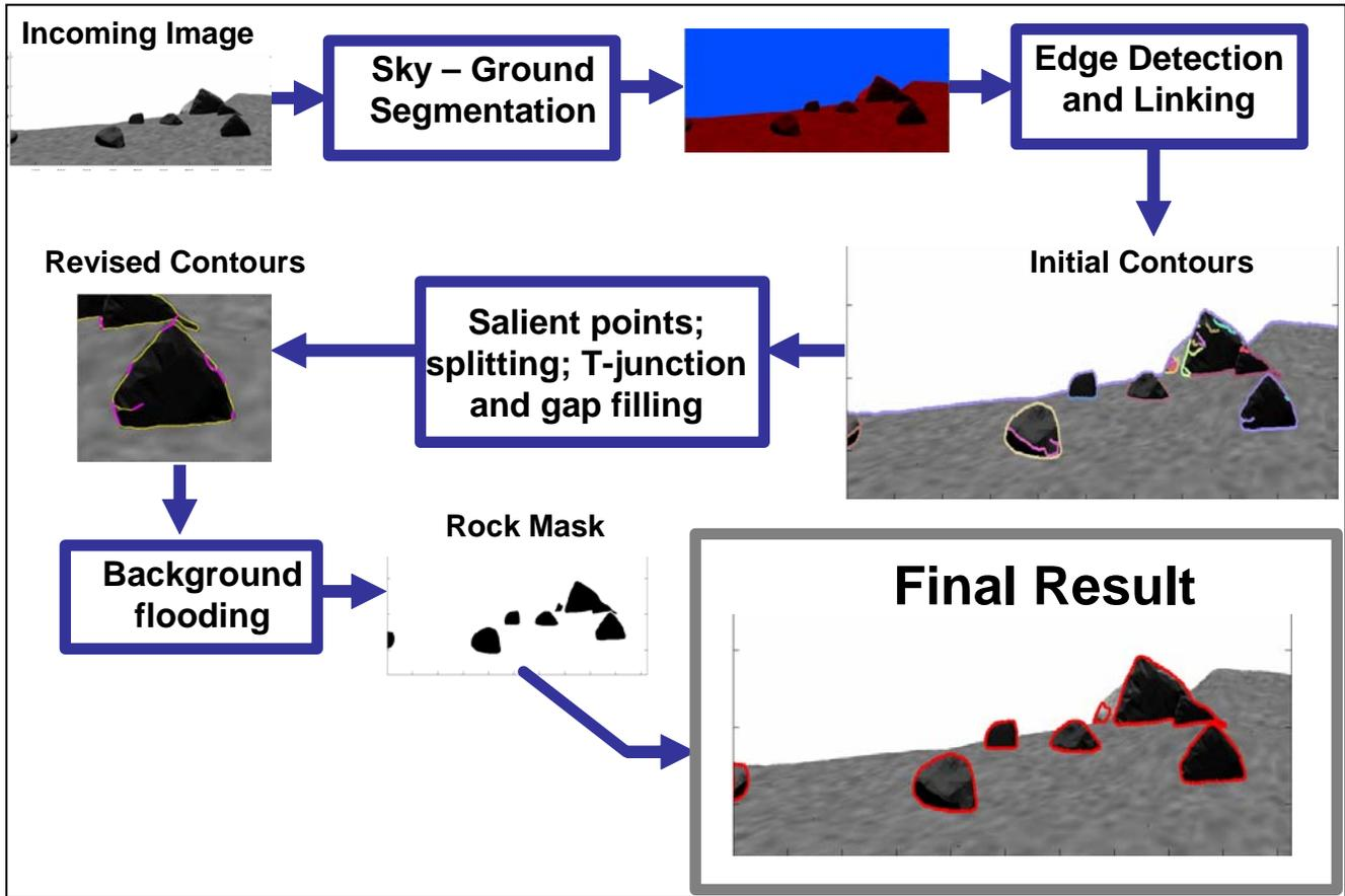
Figure 2 High-level view of the steps involved in the Rockster algorithm.
