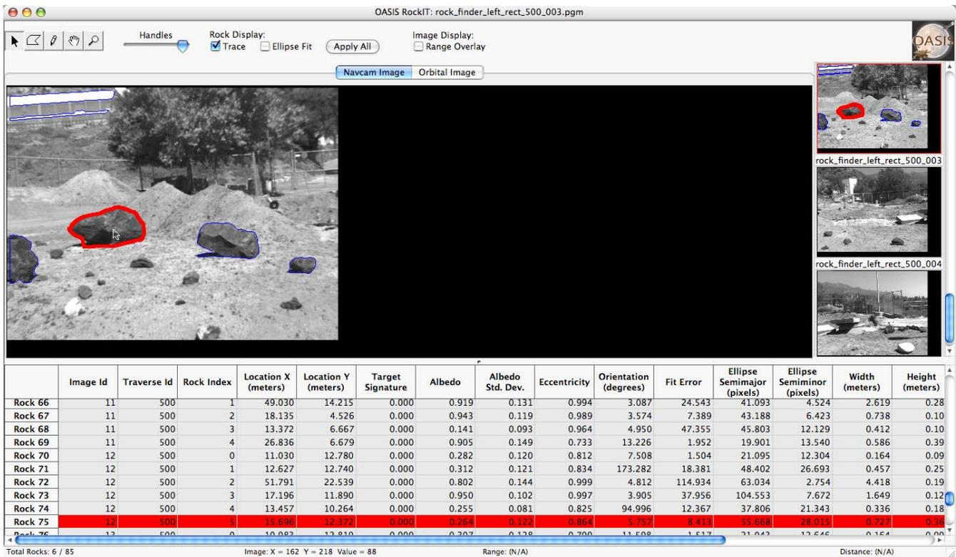
**Figure 5.** The OASIS Rock Identification Toolkit (RockIT) graphical user interface is comprised of four primary views: a main image display, a data summarization table, a scrollable list of thumbnail images (collected along a rover traverse), and an overhead map display (not shown; see Figure 6). An OASIS rock detection result is highlighted in the three views.
