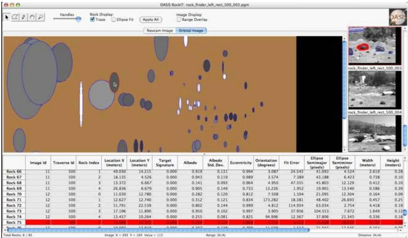
**Figure 6.** The same rock highlighted in Figure 5 is shown on the overhead map view. Rocks on the maps are represented as colored ellipses. Each ellipse is centered at the (x, y) location of the rock (z is omitted for this simple 2D map). The ellipse major and minor axes are functions of the rock’s size, and the ellipse is colored (filled) according to the rock’s average albedo.
