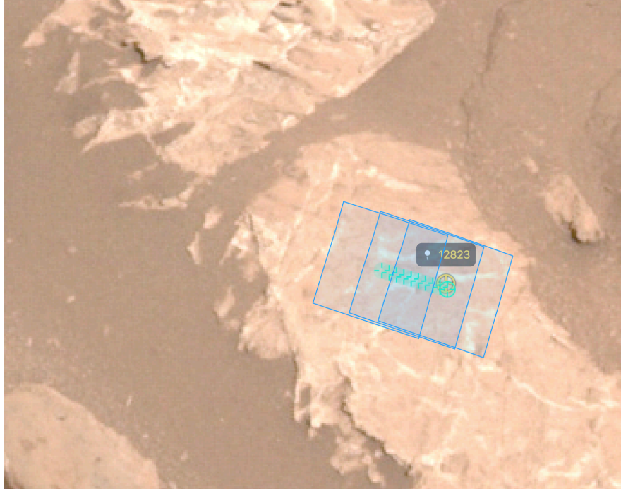
Figure 2 - Example of targeting a rock feature with SuperCam using visualization of the post-drive NavCam images and a projection of the SuperCam LIBS/VISIR points (green crosses) and RMI images (blue frames). The point 12823 is a selected rock position for targeting planning; its number is merely for identification during planning.
