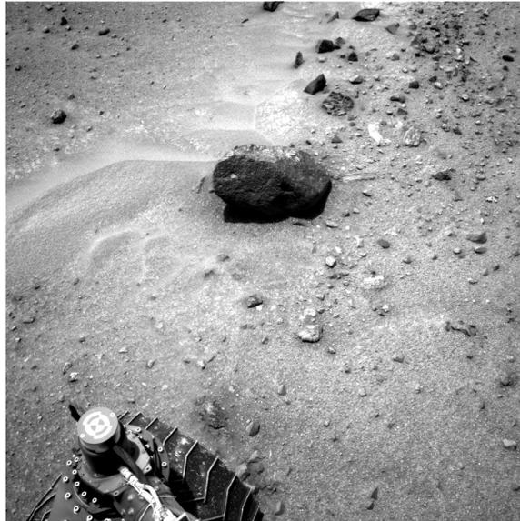
Figure 41: This NavCam image taken after the Sol 963 drive shows the nearby large rock that autonomous navigation deemed a hazard and stopped the drive early (NASA/JPL-Caltech).
