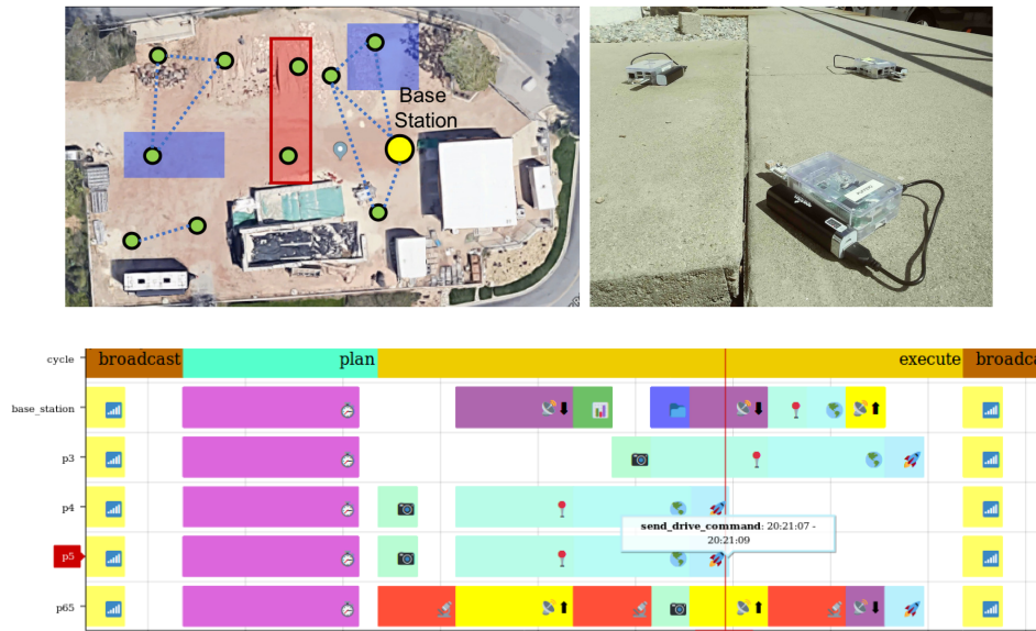
Fig. 5. Illustrative scenario in the Mars Yard at JPL (top left), pictures of the hardware nodes (top right), and one scheduled timeline (bottom). Timelines represent the operational cycle and the task allocation. Communication links can be disabled to test system adaptation and relocation of tasks. RVIZ view provides vehicle positioning and network topology information.
