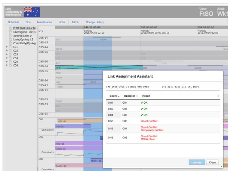
Figure 5: The link assignment assistant illustrating options for an unassigned track. Valid options are scored, and infeasible choices have a clear explanation of the conflict(s).
