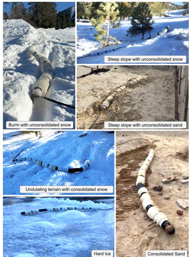
Fig. 1: The Exobiology Extant Life Surveyor (EELS) robot traversing over mobility-stressing extreme terrains
