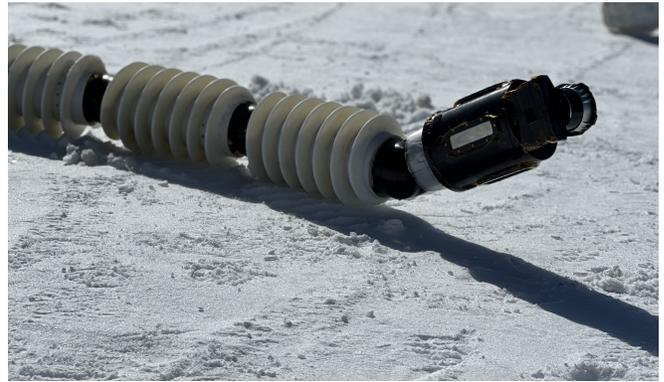
Fig. 2: The EELS exteroceptive sensor suite containing a 3D LiDar, 4x stereo pairs, and an IMU).
