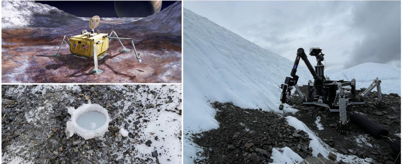
**Fig. 1** An artistic depiction of the Europa Lander is shown top left. Photographs of a Prototype Europa Lander, shown on the right, and a collected sample, shown bottom left, were taken during a field test in Alaska. The field test used our autonomy software to collect the sample, respond to off-nominal events, and communicate the data to a ground station. This test demonstrated the capabilities of our autonomous system in a real-world environment. (Images courtesy NASA/JPL-Caltech.)
