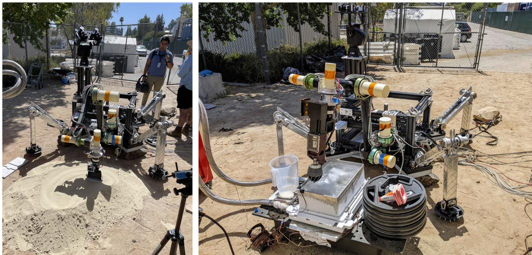
Fig. 16 Prototype Lander used during operational readiness test.
