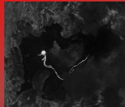
Figure 2. Ratio of Band 3/Band 4 SkySat data to enhance the hottest pixels in the scene.
