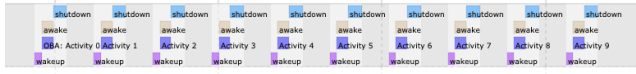
Figure 5: Sawtoothing , where each activity has its own wakeup, awake, and shutdown, occurs at low incoming SOC.
