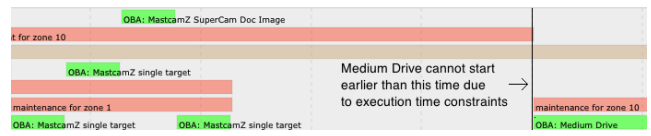
(c) In the Medium Drive Sol Type, the Medium Drive has an execution time constraint that prevents it from being scheduled earlier.
