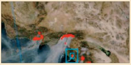
Figure A. Active fire alerts for the October 2003 Southern California fires. Red indicates active fires. The light blue box illustrates the background region used in the relative threshold detection.
