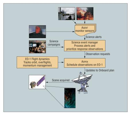
Figure 3. Sensorweb response, showing how automated retasking elements work together.
