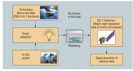
Figure 2. Sensorweb event detection and response architecture.
