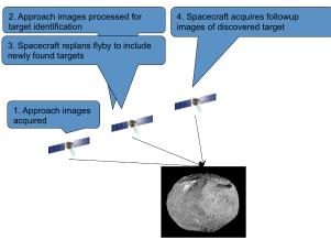
Figure 3: Onboard Autonomous Target Detection, Prioritization, and Response.
