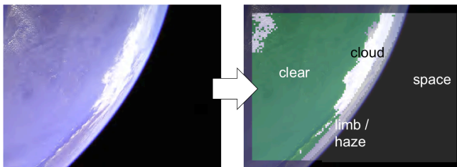
Figure 2: TextureCam image analysis uses a random forest model to classify image pixels. This simple scene required 29 seconds to classify onboard.
