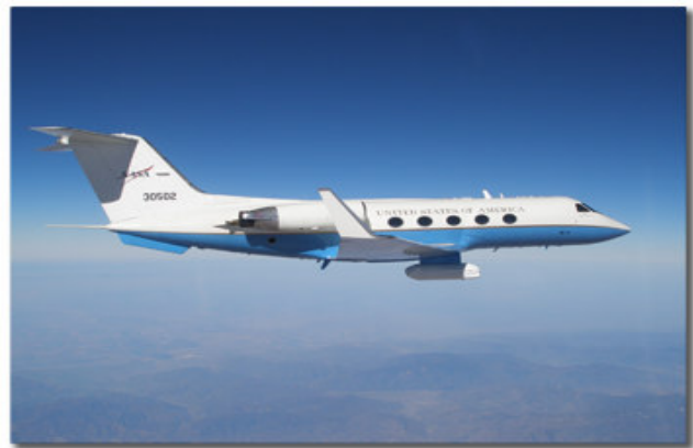
Figure 7. SAR instrument on a Gulfstream Jet, courtesy http://uavsar.jpl.nasa.gov
