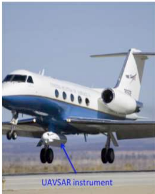
Figure 3: The UAVSAR aircraft. Note the radar mounted in the pod directly underneath the fuselage
