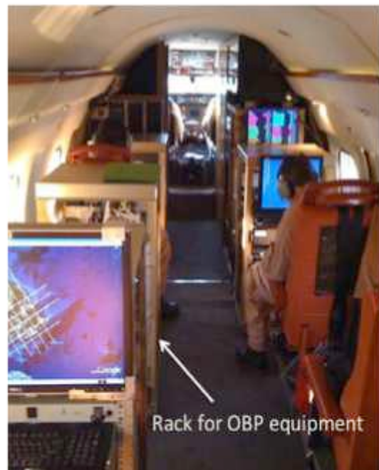
Figure 4: The interior of the UAVSAR aircraft. The rack to the left of the aisle is the rack for the onboard processing equipment.
