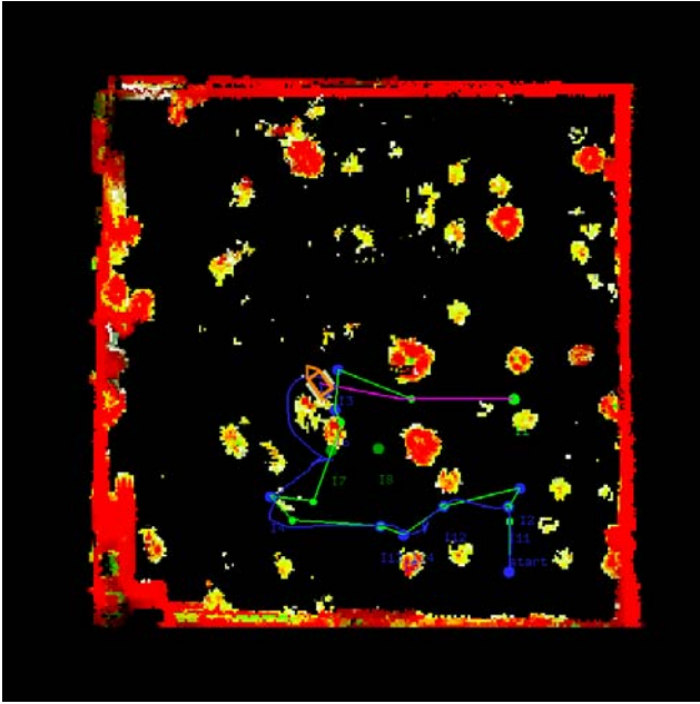
Figure 4: Sample plan shown in the Grid Visualization Tool (GriViT). Green lines show the planned path of the rover; blue lines shown the real path; and pink lines show the path that is currently executing.
