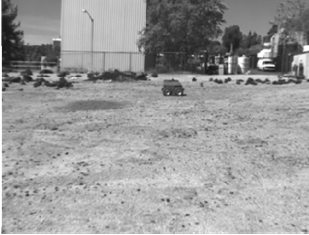
Figure 5. Dust-devil detection result taken during an atmospheric event demonstration in JPL Mars Yard. An ATRV Jr. robot was used to create dust-devil like motion. In this scenario, the motion was detected in a series of FIDO rover navigation camera images. One example from such a series is shown on the left and on the right is a snapshot of the detection result showing the area where movement was detected.
