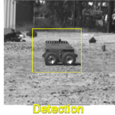
Figure 5. Dust-devil detection result taken during an atmospheric event demonstration in JPL Mars Yard. An ATRV Jr. robot was used to create dust-devil like motion. In this scenario, the motion was detected in a series of FIDO rover navigation camera images. One example from such a series is shown on the left and on the right is a snapshot of the detection result showing the area where movement was detected.
