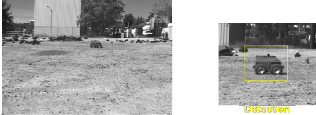
Figure 5. Dust-devil detection result taken during an atmospheric event demonstration in JPL Mars Yard. An ATRV Jr. robot was used to create dust-devil like motion. In this scenario, the motion was detected in a series of FIDO rover navigation camera images. One example from such a series is shown on the left and on the right is a snapshot of the detection result showing the area where movement was detected.
