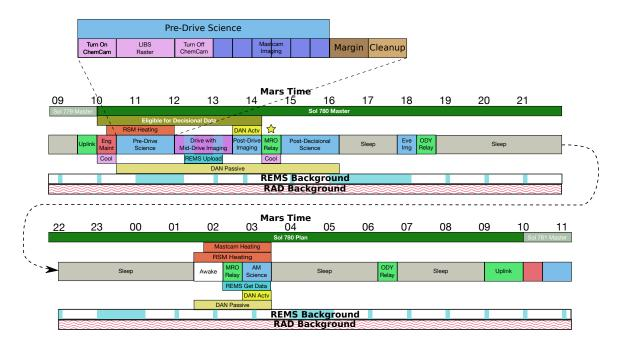
Figure 4: Example sol in the life of the rover.
