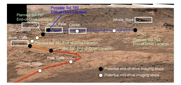
Figure 16: Curiosity's planned route for Pahrump Hills Walkabout Pass 1 at start of Sol 785 planning.
