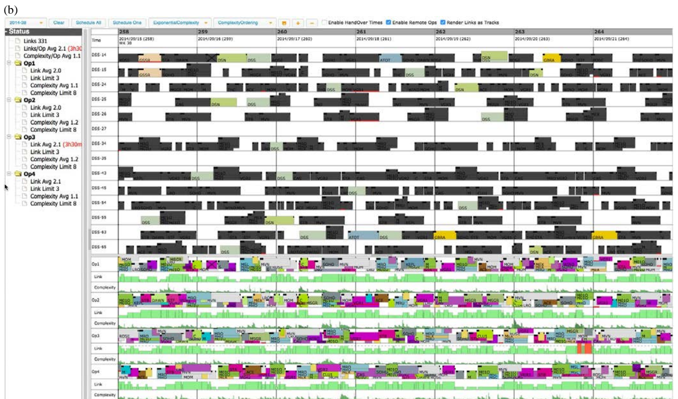
Fig. 3: Screenshots of prototype link complexity assignment GUI. (a) the original schedule with no assignments; (b) after running the complexity-based scheduling algorithm: the operator timelines at the bottom represent the workloads for a hypothetical four operators, scheduling three links apiece.
