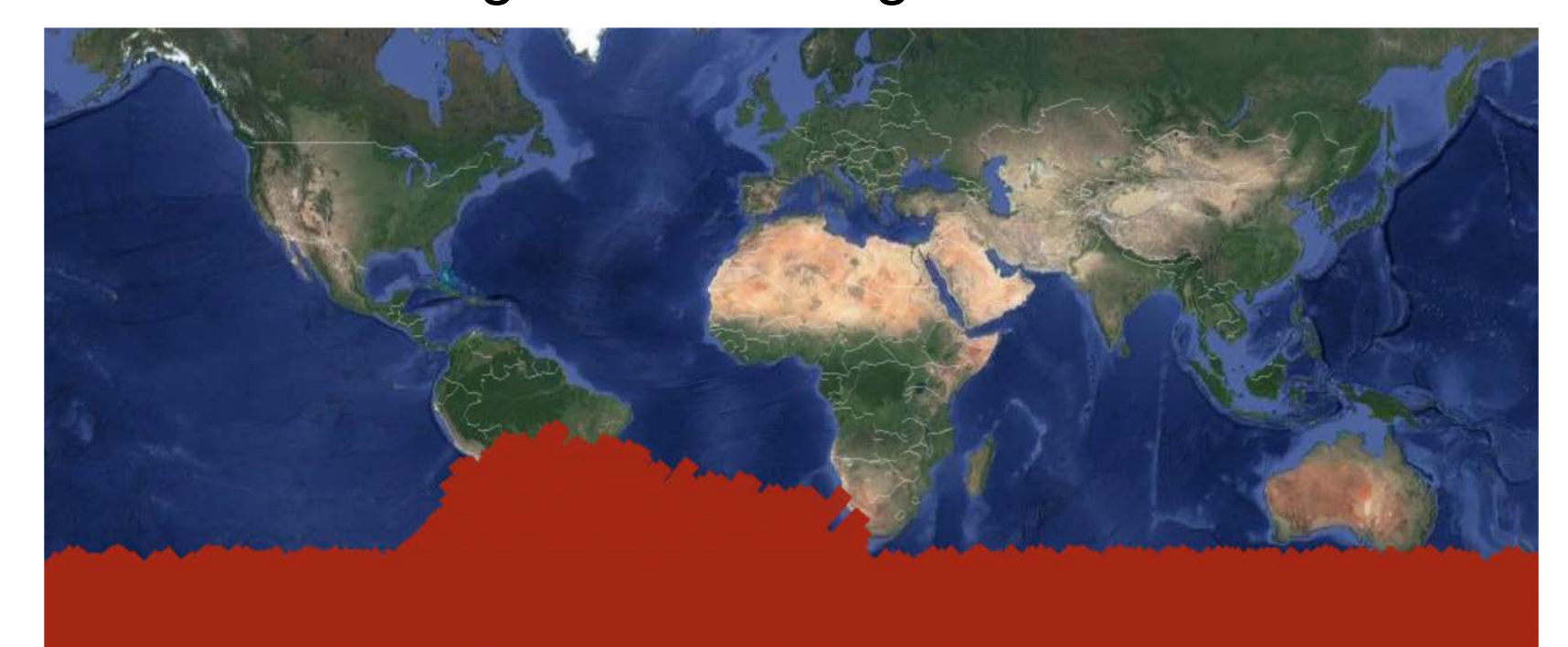
Regions where the MSU needed to be powered down due to radiation
