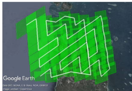
Figure 5: Milling (Knight 2014) algorithm (connected by white line) and footprints (green grid). The division causes excessive overlap and some s...
